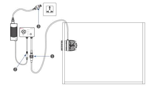
**Attention**:Before starting the pump, please ensure that livestock are not near the pump.
